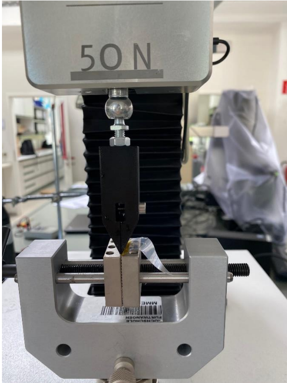
Figure II: Tensile testing machine with optimized fixture.
