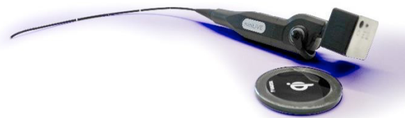
Figure 12: MiniLiVE endoscope in its latest development version. The current version of the hand piece.
