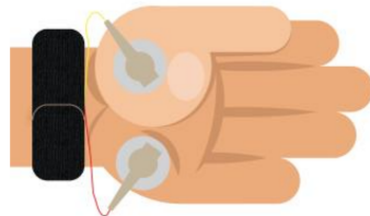
Figure 1. Graphic illustration of the EDA sensor strap and electrode placement on the non-dominant hand of the subject.
