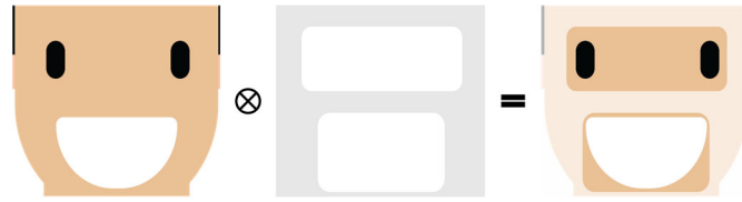
Figure 5. Graphical illustration of the mask-image fusion output of the model input layer. Original pre-processed image input ( left ), pre-defined binary mask weighted with \alpha ( middle ), and output of model input layer ( right ).
