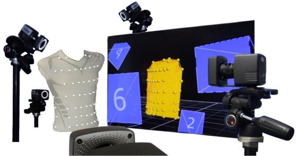
Figure 1. Schematic of the MoCap system. Five of the nine infrared cameras, the compression shirt with MoCap markers and the representation of the MoCap markers by the Vicon Systems on a screen. Figure published in [3].
