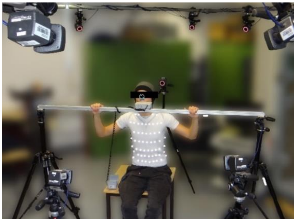
Figure 3. Measurement setup: A subject wearing the compression shirt with MoCap markers, breathing through the spirometer, which was fixed on the rigid mount and surrounded by the MoCap cameras. Figure published in [3].
