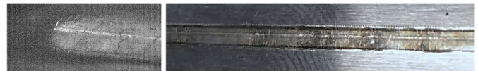
Figure 2: Weld during (left) and after (right) conduction mode laser welding at 110 J/cm (700 W, 4 m/min) with a calm melt pool
