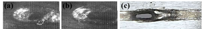
Figure 5: Keyhole formation (a) and elongation (b) at 170 J/cm (1100 W, 4 m/min) and the resulting welding defect (c)
