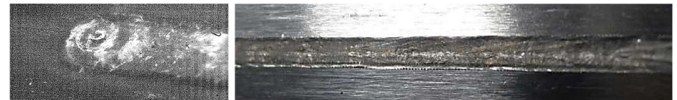
Figure 3: Weld during (left) and after (right) laser welding at 120 J/cm (800 W, 4 m/min) with a boiling melt pool
