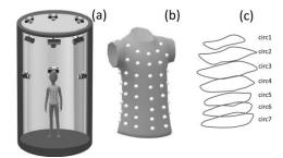
Figure 1: Sketch of the MoCap System (a) and the used compression shirt with MoCap markers (b). In (c) the circumferences are illustrated (based on the data of subject 1).
