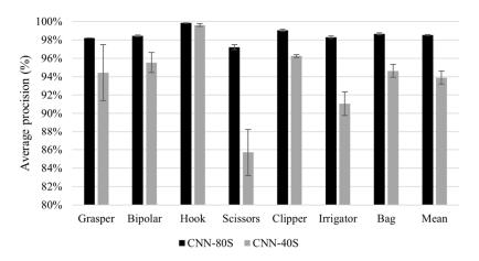
**Figure 4.** Results of generalisation to new subjects. Average precision of tool presence detection for all tools yielded by CNN-80S model (back bars) and CNN-40S model (grey bars). Note the truncated scale of the *y*-axis.
