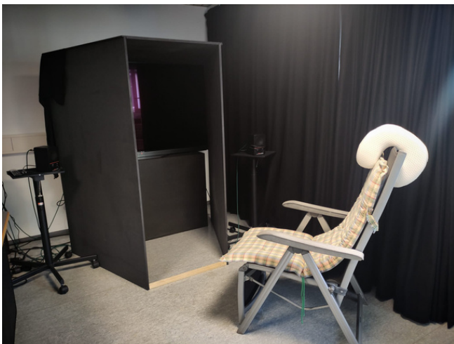
Figure 9: Setup TV box / comparison group, nearfield loudspeakers and chair (Alka et al. 2022)
