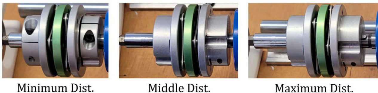
Figure 2: Distances between screw bit holder and torque sensor for the 3 cases tested.
