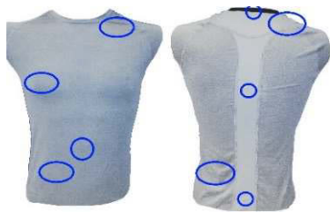
Figure 4: Areas of the shirt, containing the major information content of the system regarding respiration according to [9].
