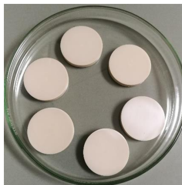
Figure 1: PEEK specimens for the determination of contact angles and surface energy.
