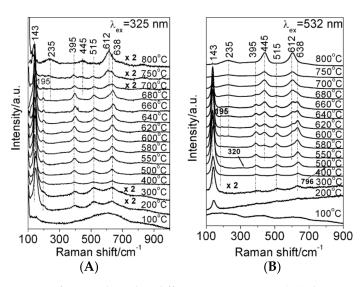
**Figure 4.** Raman spectra of  $TiO_2$  calcined at different temperatures. (**A**) The spectra were recorded with an excitation at 325 nm, (**B**) with 532 nm. Reprinted with permission from The Journal of Physical Chemistry B, reference [63]. Copyright 2006 American Chemical Society.
