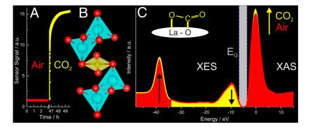
**Figure 3.** Operando spectroscopic study of  $La_2O_3CO_3$  during  $CO_2$  (10,000 ppm) sensing in 50 %r.h. at 250 °C: (**A**) Sensor signals, (**B**) schematics of the unit cell of  $La_2O_2CO_3$  (La = cyan, O = red, C = yellow) and (**C**) XES and XAS spectra before (red) and during (yellow)  $CO_2$  exposure. Figure is reprinted from reference [38].
