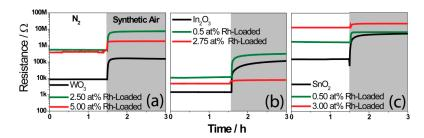
**Figure 6.** The resistances of the sensors, based on WO<sub>3</sub> (**a**),  $In_2O_3$  (**b**), and  $SnO_2$  (**c**), are shown in  $N_2$  and dry synthetic air background (80%  $N_2$  and 20%  $O_2$ ).
