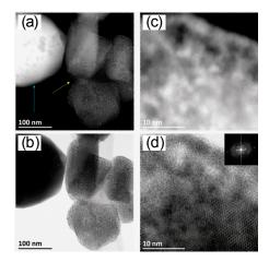
**Figure 3.** STEM images of 2.75 at.% Rh-Loaded  $In_2O_3$ . (a) STEM HAADF and (b) STEM bright-field (BF) images show two kinds of structures: low Rh-loaded (blue arrows) and high Rh-loaded (yellow arrow). (c) High-resolution (HR)-STEM HAADF and (d) HR-STEM BF images show high crystalline  $In_2O_3$  and a rich Rh layer around  $In_2O_3$ . The inset in (d) is the fast Fourier transform (FFT) of the STEM BF image.
