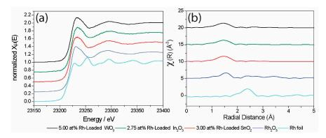
**Figure 4.** Rh K-edge X-ray absorption near-edge structure (XANES) spectra (**a**) and Fourier transform (FT)  $k^3$ -weighted extended X-ray absorption fine structure (EXAFS) spectra (**b**) of Rh-loaded sensing materials (amplitude  $\times$  2), Rh<sub>2</sub>O<sub>3</sub> reference (amplitude  $\times$  2), and Rh foil  $\left(\frac{\text{amplitude}}{2}\right)$ .
