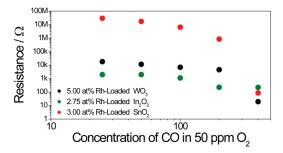
**Figure 11.** The change in resistance of the sensors during exposure to different CO concentrations in low-oxygen background, acquired during simultaneously measured X-ray absorption spectroscopy (XAS), is plotted in log-log.
