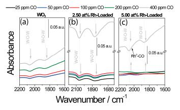
**Figure 8.** DRIFT spectra taken during exposure to different CO concentrations in low-oxygen (50 ppm O<sub>2</sub>) backgrounds for (**a**) unloaded WO<sub>3</sub> sample, (**b**) 2.50 at.% Rh<sub>2</sub>O<sub>3</sub> loaded WO<sub>3</sub>, and (**c**) 5 at.% Rh<sub>2</sub>O<sub>3</sub> loaded WO<sub>3</sub>.
