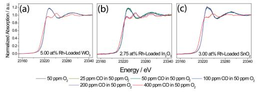
**Figure 12.** Rh K-edge XANES spectra of 5.00 at.% Rh-loaded WO<sub>3</sub> (**a**), 2.75 at.% Rh-loaded In<sub>2</sub>O<sub>3</sub> (**b**), and 3.00 at.% Rh-loaded SnO<sub>2</sub> (**c**), recorded during different CO exposures in a low-oxygen background (50 ppm O<sub>2</sub>) at 300  $^{\circ}$ C.
