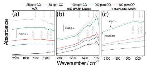
**Figure 9.** DRIFT spectra taken during exposure to different CO concentrations in low-oxygen (50 ppm O<sub>2</sub>) backgrounds for (**a**) unloaded In<sub>2</sub>O<sub>3</sub> sample, (**b**) 0.50 at.% Rh<sub>2</sub>O<sub>3</sub> loaded In<sub>2</sub>O<sub>3</sub>, and (**c**) 2.75 at.% Rh<sub>2</sub>O<sub>3</sub> loaded In<sub>2</sub>O<sub>3</sub>.
