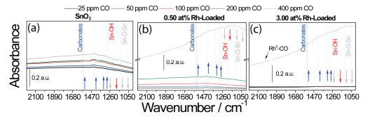
**Figure 10.** DRIFT spectra taken during exposure to different CO concentrations in low-oxygen (50 ppm  $O_2$ ) backgrounds for (a) unloaded  $SnO_2$  sample, (b) 0.50 at.%  $Rh_2O_3$  loaded  $SnO_2$ , and (c) 3.00 at.%  $Rh_2O_3$  loaded  $SnO_2$ .
