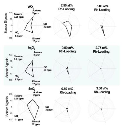
**Figure 5.** Signals of the sensors based on the different materials with various test gases in dry air at an operation temperature of 300  $^{\circ}$ C. The results are shown in a polar plot in order to highlight the general qualities of the sensors.
