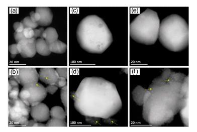
**Figure 2.** Scanning transmission electron microscopy (STEM) high-angle annular dark-field (HAADF) images of pure and Rh-loaded clusters on three different supports: SnO<sub>2</sub> (**a**) pure and (**b**) 3.00 at.% Rh-loaded SnO<sub>2</sub>; In<sub>2</sub>O<sub>3</sub> (**c**) pure and (**d**) 2.75 at.% Rh-loaded In<sub>2</sub>O<sub>3</sub>; WO<sub>3</sub> (**e**) pure and (**f**) 5.00 at.% Rh-loaded WO<sub>3</sub>. Yellow arrows show the Rh<sub>2</sub>O<sub>3</sub> particles and clusters.
