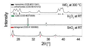
**Figure 1.** X-ray diffractograms taken of the sensitive layer on the sensors ( $SnO_2$  and  $In_2O_3$  at room temperature;  $WO_3$  was recorded on a heated sensor). The reference patterns are from the Crystallography Open Database.
