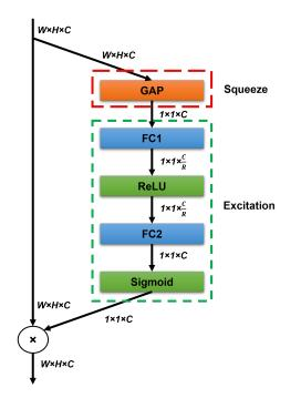
Figure 2. Squeeze-and-excitation attention module architecture.
